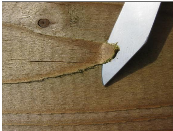
Jaarring kan delamineren (raising grain)
